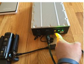
12. Press Record on the front of the T100. The Record LED should turn **ORANGE**. *NOTE: If your Orange LED is blinking, check the camera/cables for a loose connection*.
