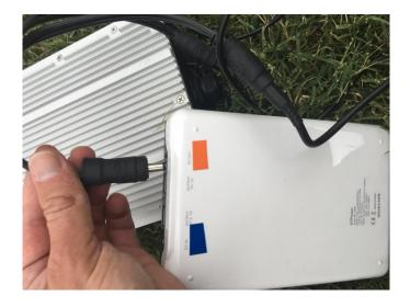
Step # 2 -- Connect the BLACK end of Split Power Cable to the DC IN port on the T100.
