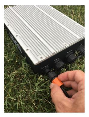
Step # 3 -- Power ON your Camera. Using 6' HDMI cable or 25' HDMI cable and appropriate adapter (micro HDMI or mini HDMI), connect T100 HDMI In port to the camera as shown.
