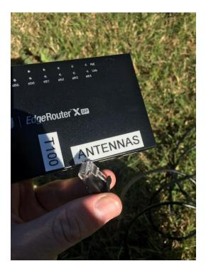
Step # 4 – Connect an Ethernet cable from T100 LAN port to the EdgeRouter port labeled T100 as shown below.
