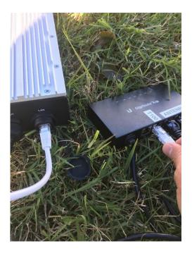
Step # 5 – Plug EdgeRouter into power source (into wall w/ extension cord or battery w/ AC plugin)
