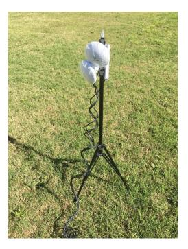
Step #2 - Attach (2) white antennas to access point.
