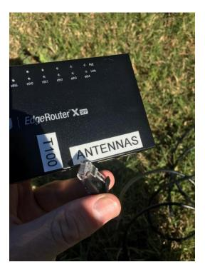
Step # 4 – Connect an Ethernet cable from T100 LAN port to the EdgeRouter port labeled T100 as shown below.
