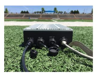
STEP 1.E: Connect BLACK Coaxial Cable to Long Range Antenna (LRA) & the Router. NOTE: Coaxial Cable should be screwed into router antenna port closest to the power outlet.
