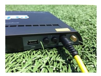
STEP 1.D: Connect GRAY Ethernet Cable from LAN port on T100 to PORT 1 on the Router.
