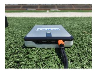
STEP 1.B: Connect BLACK end of Split Power Cable to the DC IN port on the T100.
